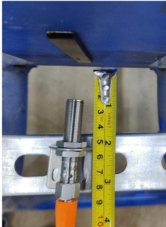
Figure 119: Mounting Proximity Sensor Assembly (Example)
