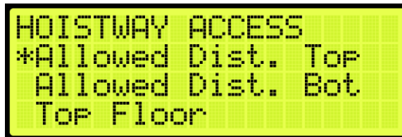
Figure 400: HOISTWAY ACCESS – Allowed Distance Top
