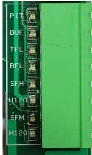
Figure 19: Safety String Input Connector
