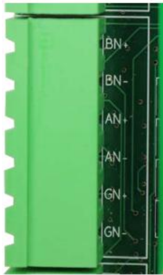
Figure 14: CAN 1,2,3 Network Connector
