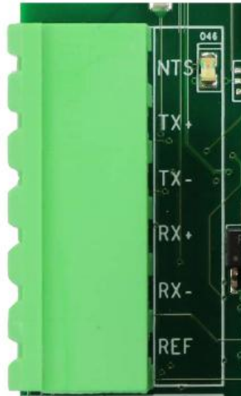
Figure 12: Drive Communication Connector
