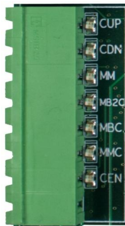
Figure 18: 24 VDC Monitoring System Connector
