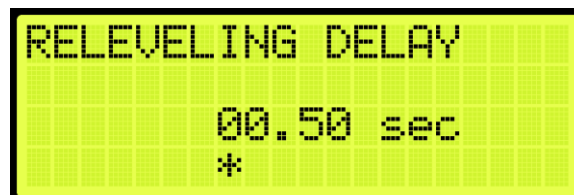
Figure 156: RELEVELING DELAY Menu
