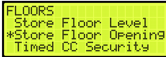
Figure 163: FLOORS Menu – Short Floor Opening
