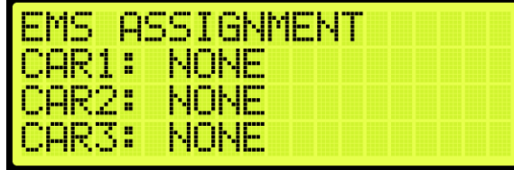
Figure 665: EMS STATUS Menu – No Cars Assigned
