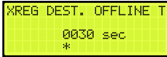
Figure 699: XREG DESTINATION OFFLINE TIMEOUT Menu
