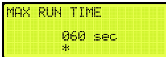
Figure 435: MAXIMUM RUN TIME Menu
