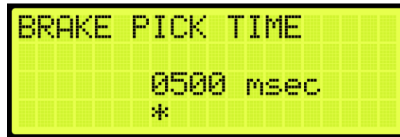
Figure 89: BRAKE PICK TIME Menu
