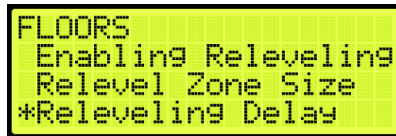
Figure 254: FLOORS Menu – Releveling Delay
