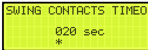
Figure 359: SWING CONTACTS TIMEOUT Menu
