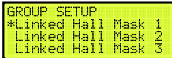
Figure 392: GROUP SETUP Menu – Linked Hall Mask
