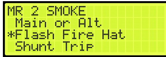
Figure 618: MR 2 SMOKE Menu – Flash Fire Hat
