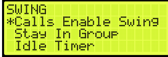
Figure 491: SWING Menu – Calls Enable Swing
