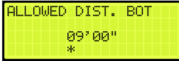
Figure 418: ALLOWED DISTANCE – BOTTOM Menu
