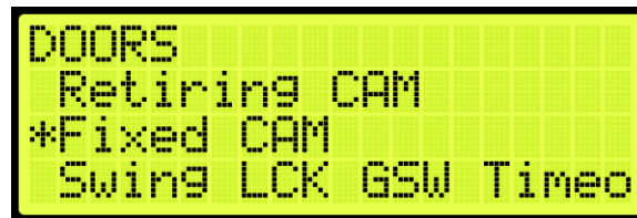
Figure 354: DOORS Menu – Fixed CAM
