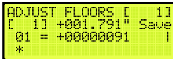
Figure 233: ADJUST FLOORS Menu – Too Low
