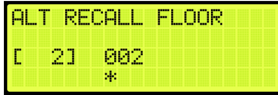
Figure 566: ALT RECALL FLOOR Menu
