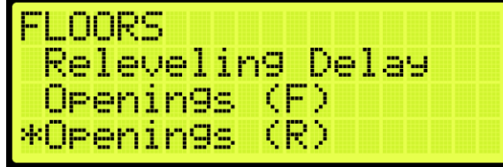
Figure 256: FLOOR Menu – Openings
