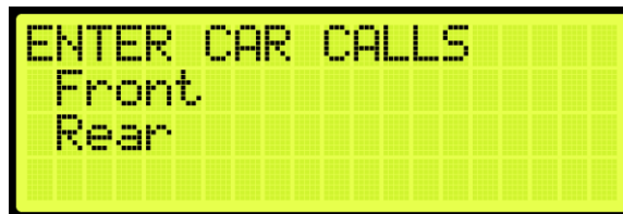
Figure 711: ENTER CAR CALLS Menu – Front or Rear
