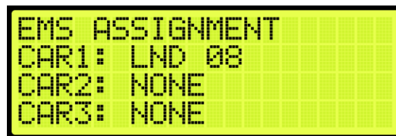
Figure 664: EMS STATUS Menu – Car 1 Assigned
