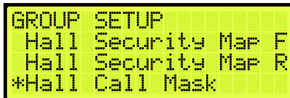
Figure 390: GROUP SETUP Menu – Hall Call Mask
