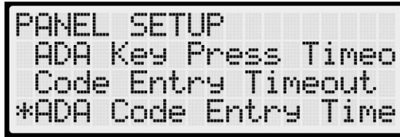
Figure 21: PANEL SETUP Menu – ADA Code Entry Timeout
