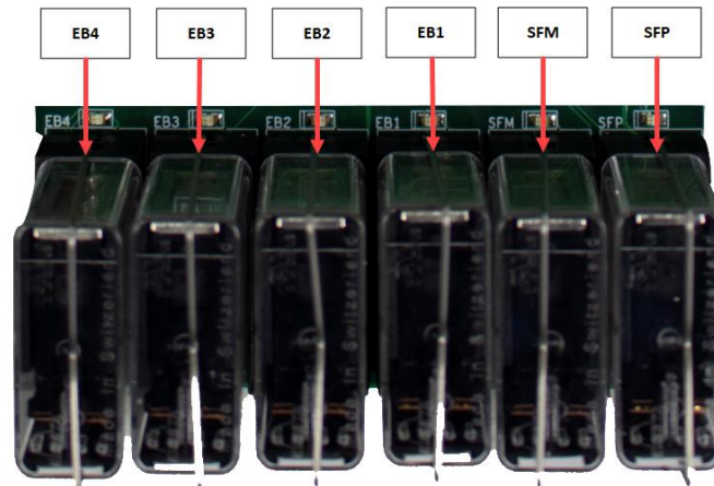
Figure 23: MR Board SR3032 Safety Relays
