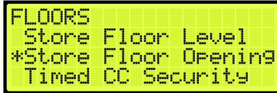
Figure 161: FLOORS Menu – Short Floor Opening
