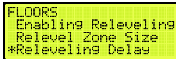
Figure 153: FLOORS Menu – Releveling Delay
