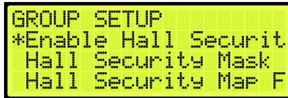
Figure 282: MISCELLANEOUS Menu – Enable Hall Security
