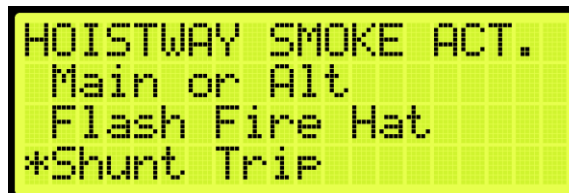
Figure 541: HOISTWAY SMOKE ACTION Menu – Shunt Trip
