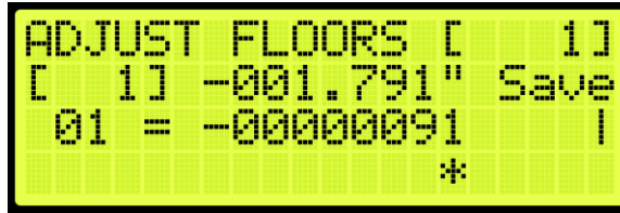
Figure 133: ADJUST FLOORS Menu – Too High
