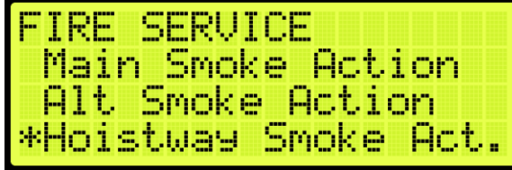
Figure 579: FIRE SERVICE Menu – Hoistway Smoke Action
