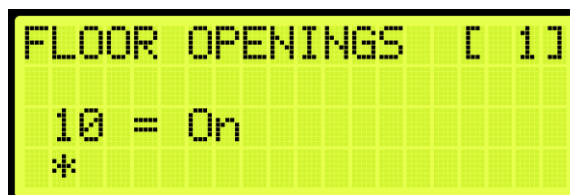
Figure 286: FLOORS OPENINGS (Rear) Menu
