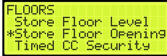
Figure 260: FLOORS Menu – Short Floor Opening
