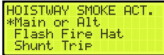
Figure 580: HOISTWAY SMOKE ACTION Menu – Main or Alt
