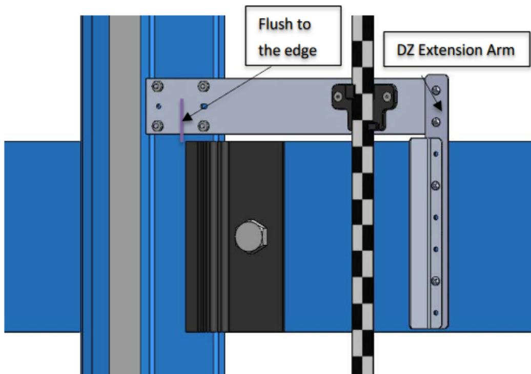
Figure 73: Tape Clip Assembly Alignment
