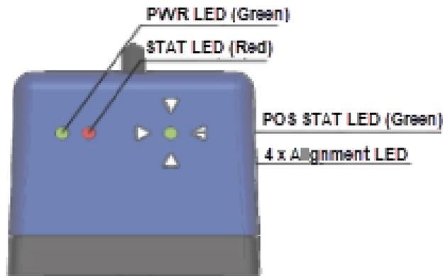
Figure 84: Camera LEDs
