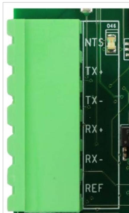
Figure 11: Drive Communication Connector
