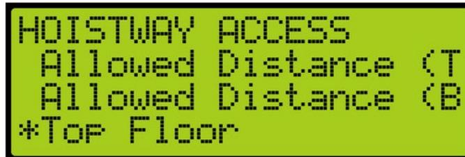
Figure 168: HOISTWAY ACCESS – Top Floor
