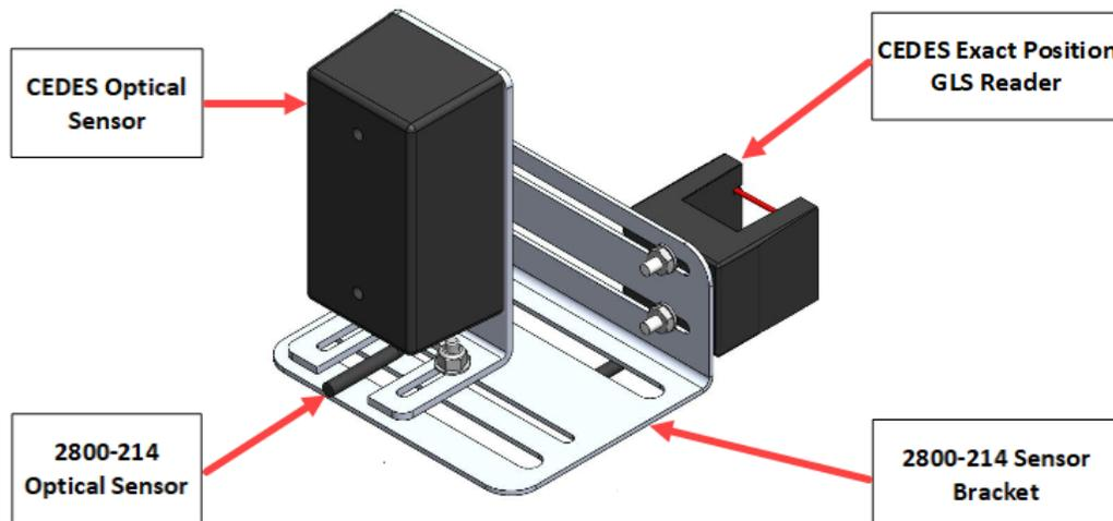
Figure 64: Sensor Assembly
