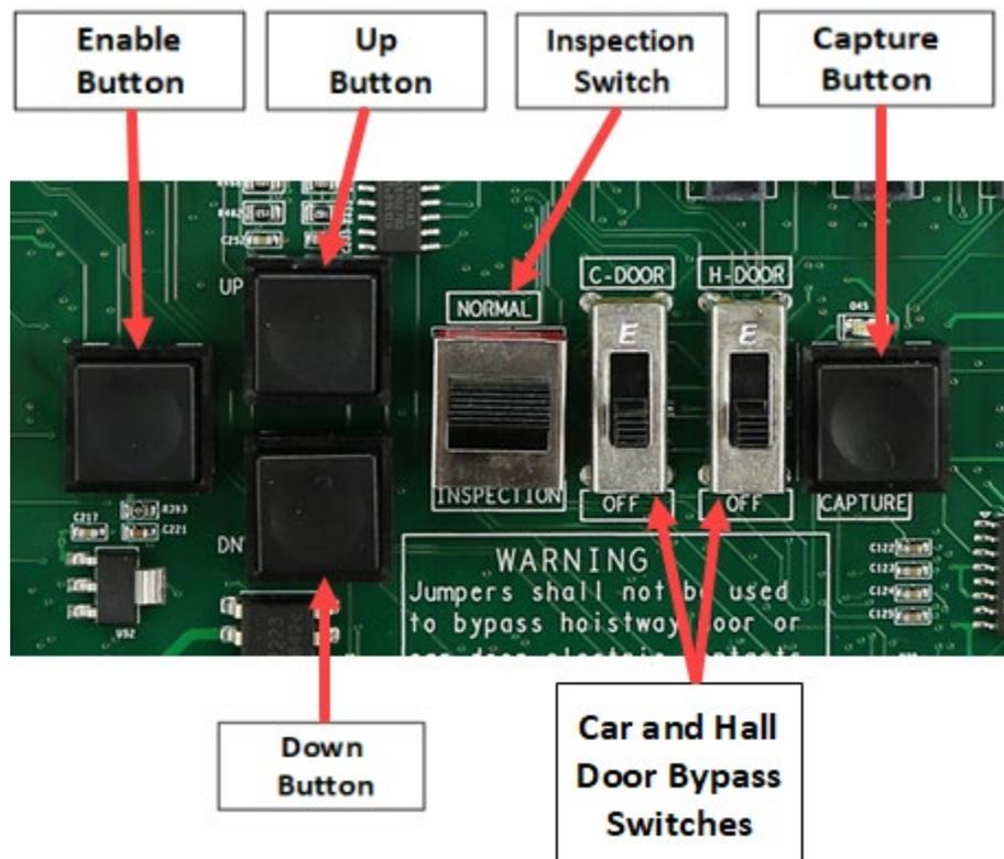
Figure 21: MR Board SR3032 Inspection Control
