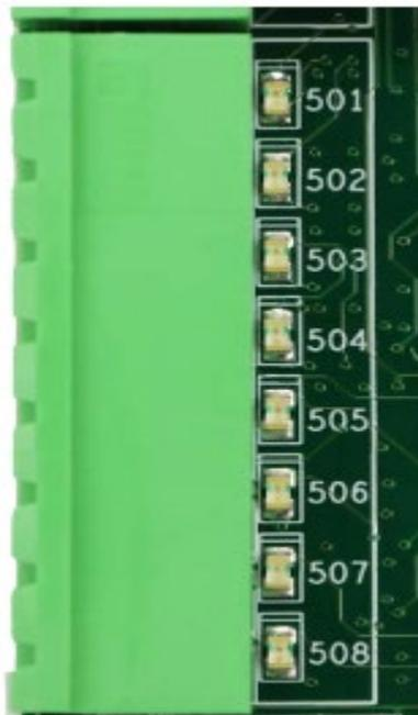
Figure 15: 24 VDC Input Connector
