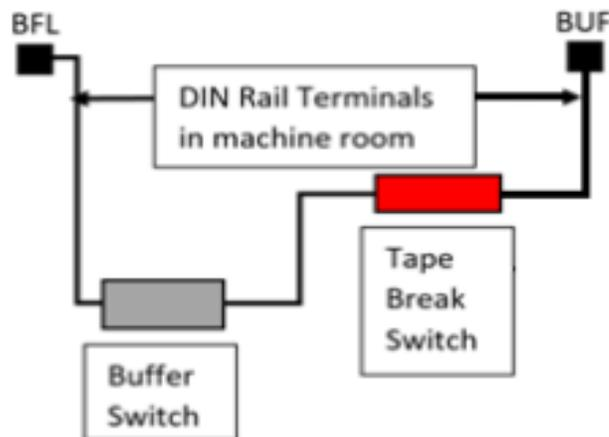
Figure 80: Emergency Tape Break Switch in Series with Buffer Switch
