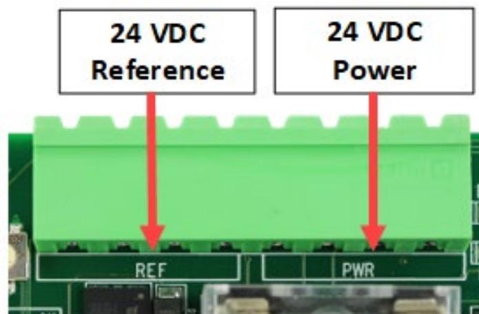
Figure 9: 24 VDC Connector
