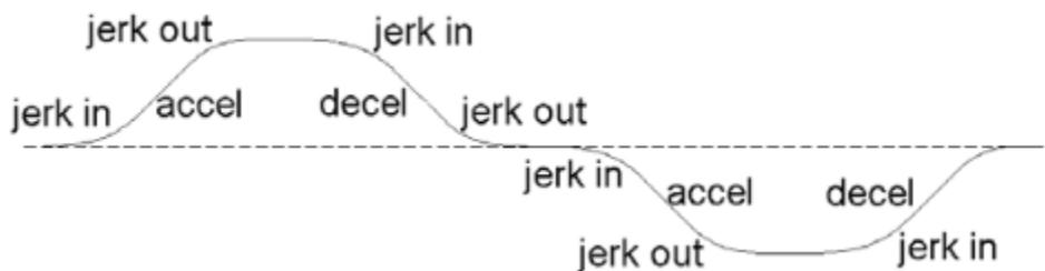
Figure 51: Graphical Representation of an S-Curve
