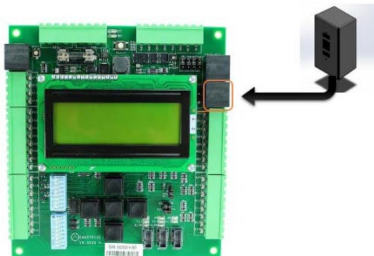
Figure 83: RJ45 Connection
