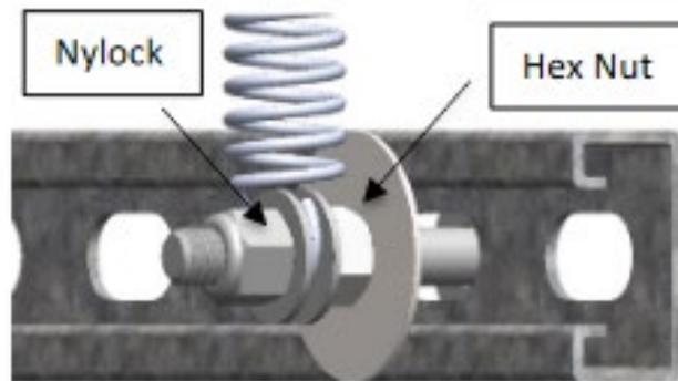
Figure 79: Hardware to Lower Tape Mount Assembly
