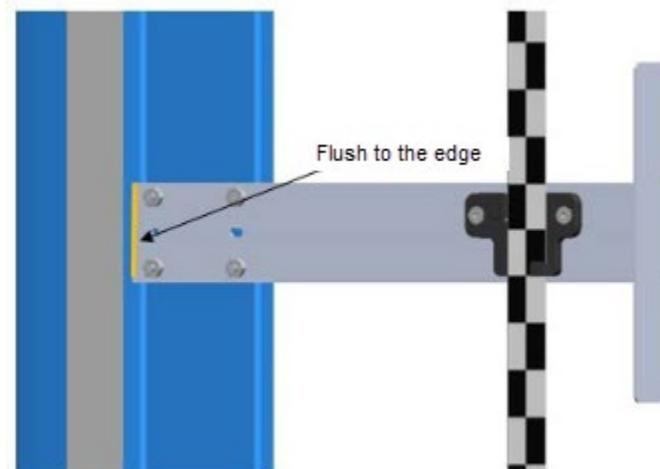
Figure 72: Tape Clip Assembly Alignment
