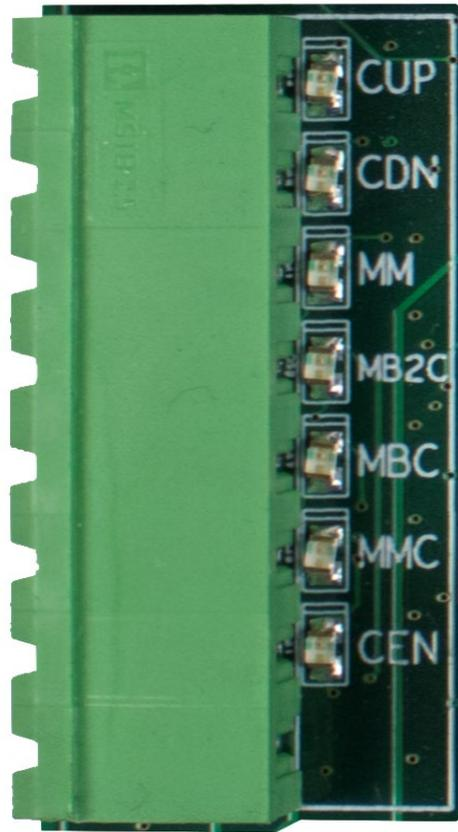
Figure 17: 24 VDC Monitoring System Connector
