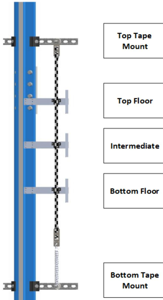
Figure 74: Tape Mount Assembly
