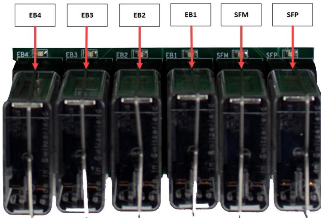
Figure 22: MR Board SR3032 Safety Relays
