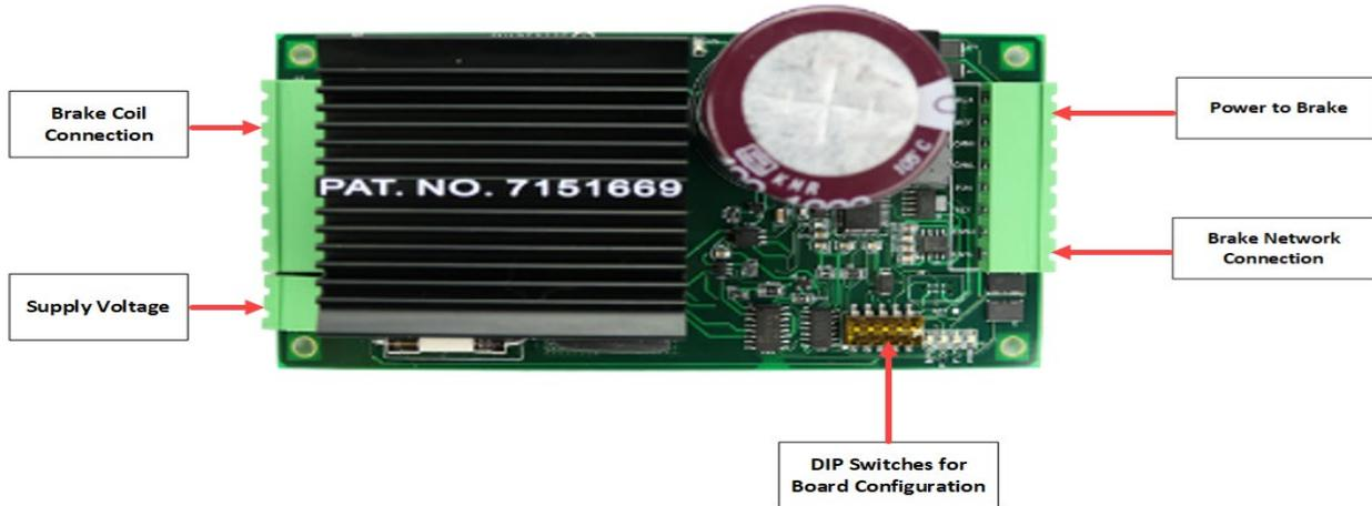
Figure 26: Brake Board SR3038
