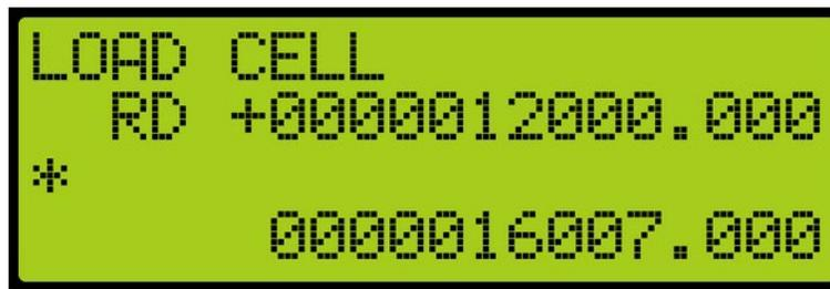
Figure 200: LOAD CELL Menu – New Load Cell Value
