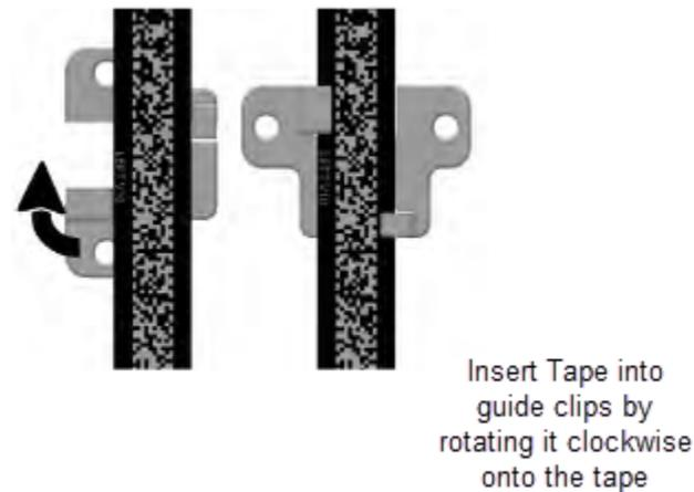
Figure 69: Tape Clip Insertion
