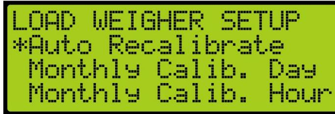
Figure 244: LOAD WEIGHER SETUP Menu – Auto Recalibrate
