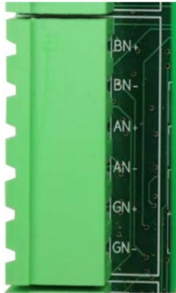
Figure 13: CAN 1,2,3 Network Connector
