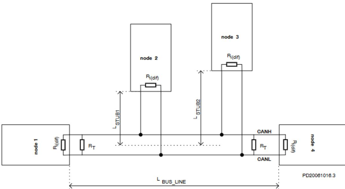
Figure 151: Standard CAN Bus<sup>1</sup>
