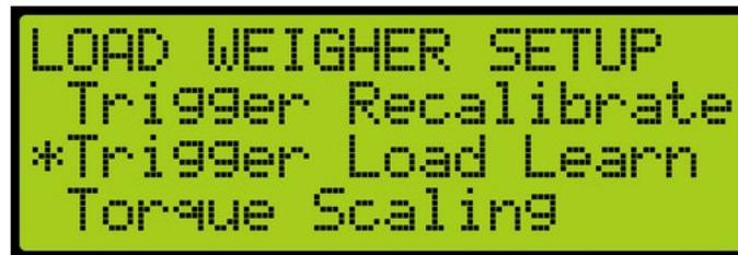
Figure 218: LOAD WEIGHER SETUP Menu – Trigger Load Learn
