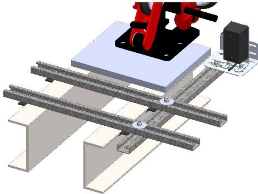
Figure 67: Alternate Unistrut Installation
