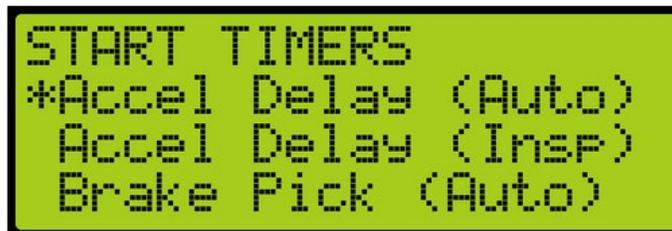
Figure 227: START TIMERS Menu – Accel Delay (Auto)
