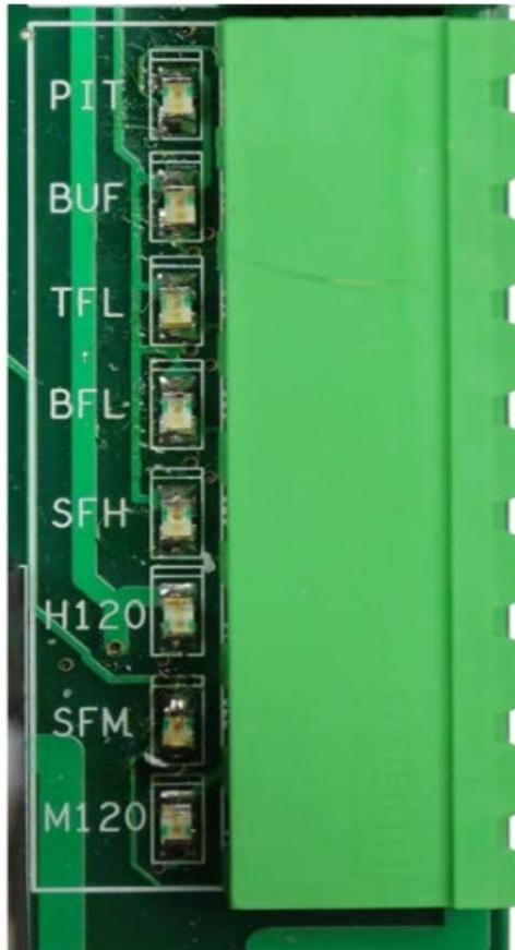
Figure 18: Safety String Input Connector
