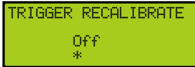
Figure 217: TRIGGER RECALIBRATE Menu – Off
