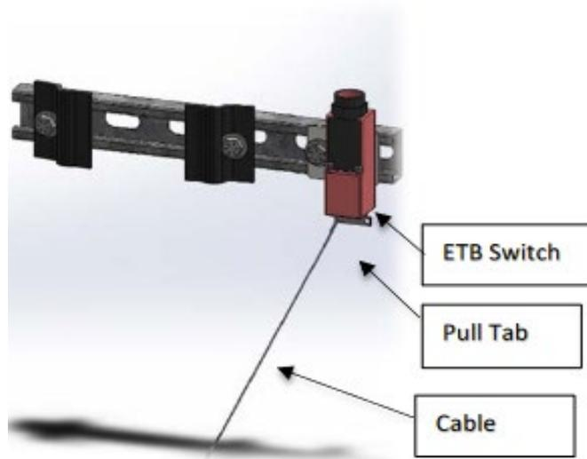
Figure 82: Emergency Tape Break Switch
