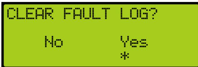
Figure 254: CLEAR FAULT LOG Menu – Clear Log
