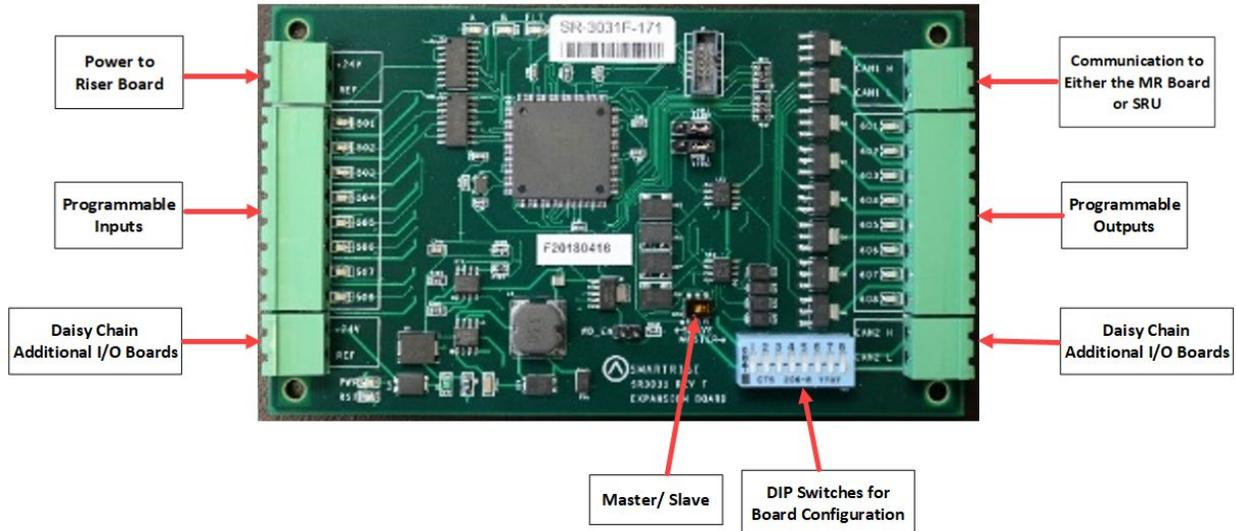
Figure 24: IO Board/Riser Board SR3031
