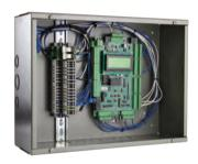
Car Top Controllers The Car Top Controller manages part of the safety logic. It connects to the top of the car components and the Traveler Cable.
