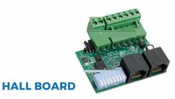
Provides a serial connection to hall fixtures. It turns Top & Bottom Access Switches, Fire Service Switches, Hall Buttons & Lanterns, and Medical Service Switches into networked devices.
