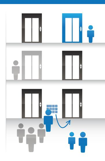
Passengers are grouped based on destination. This reduces the number of stops and the overall travel time.
