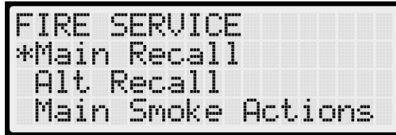
Figure 265: FIRE SERVICE Menu – Main Recall, Alt Recall, Main Smoke Actions
