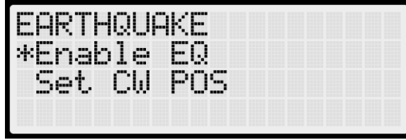
Figure 281: EARTHQUAKE Menu – Enable EQ, Set CW Pos
