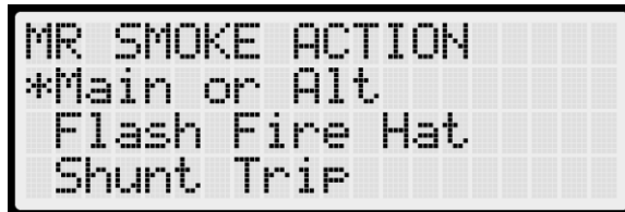
Figure 272: MR SMOKE ACTION Menu – Main or Alt, Flash Fire Hat, Shunt Trip
