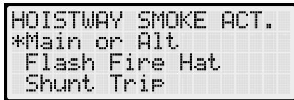
Figure 271: HOISTWAY SMOKE ACTION Menu – Main or Alt, Flash Fire Hat, Shunt Trip
