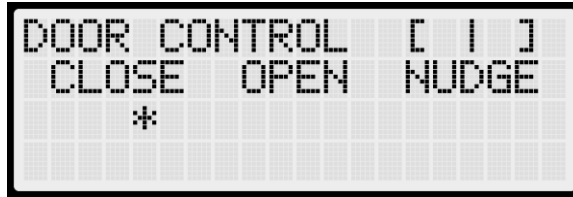
Figure 367: Enter Door Command Menu (Front Doors Only)
