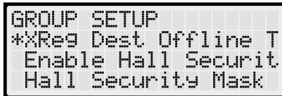
Figure 301: GROUP SETUP Menu – XReg Destination Offline Timeout, Enable Hall Security, Hall Security Mask
