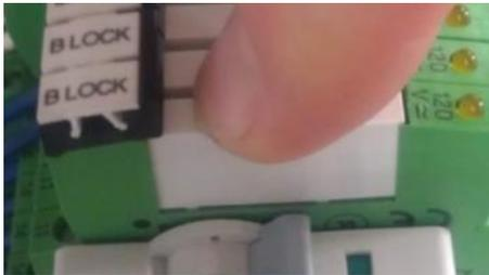
**\*\* NOTE:** If the relay you're replacing is burnt out, has been arcing or is missing a pin, you should replace the whole relay/base assembly. This will eliminate any damage done to the base from the relay terminals.
