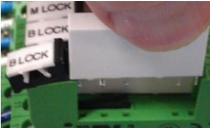
3. Re-install the relay the same way making sure you don't bend any pins when inserting it into the base. Pushing down on the relay will snap the black tab back into the locking position.
