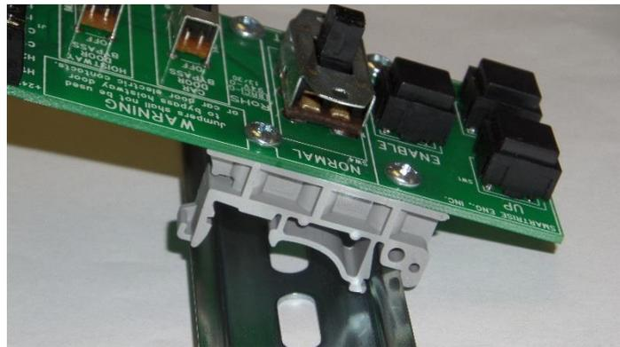
7. Rotate the new board down onto the rail and snap it into place.
