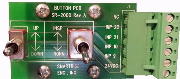
4. Remove the Inspection board from the rail by reaching behind the plug side and prying up on the two grey tabs that attach it to the rail.
