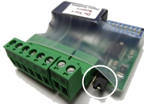
Termination Jumper - **Last** HCB in series – farthest HCB from machine room
