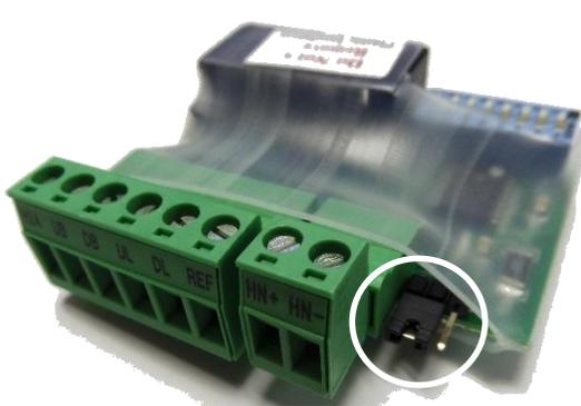
Termination Jumper - All HCB's in series will have the jumper placed this way.
