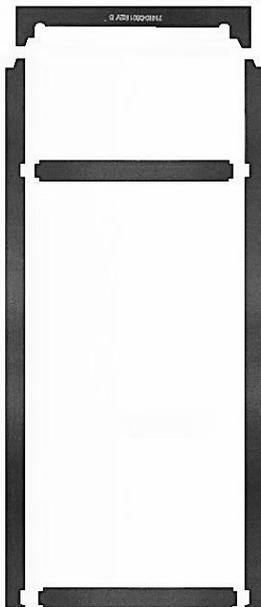
There are 5 gaskets that need to be installed on the backside of the air conditioner unit. The orientation of the gaskets on the back of the unit is as pictured. The tabs of the smaller cross pieces go into the notches on the longer side pieces. When installed correctly the gaskets should provide a consistent seal all the way around the enclosure face with no gaps to allow cold air to escape.
