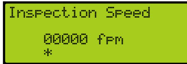
Figure 13: Inspection Speed Menu
