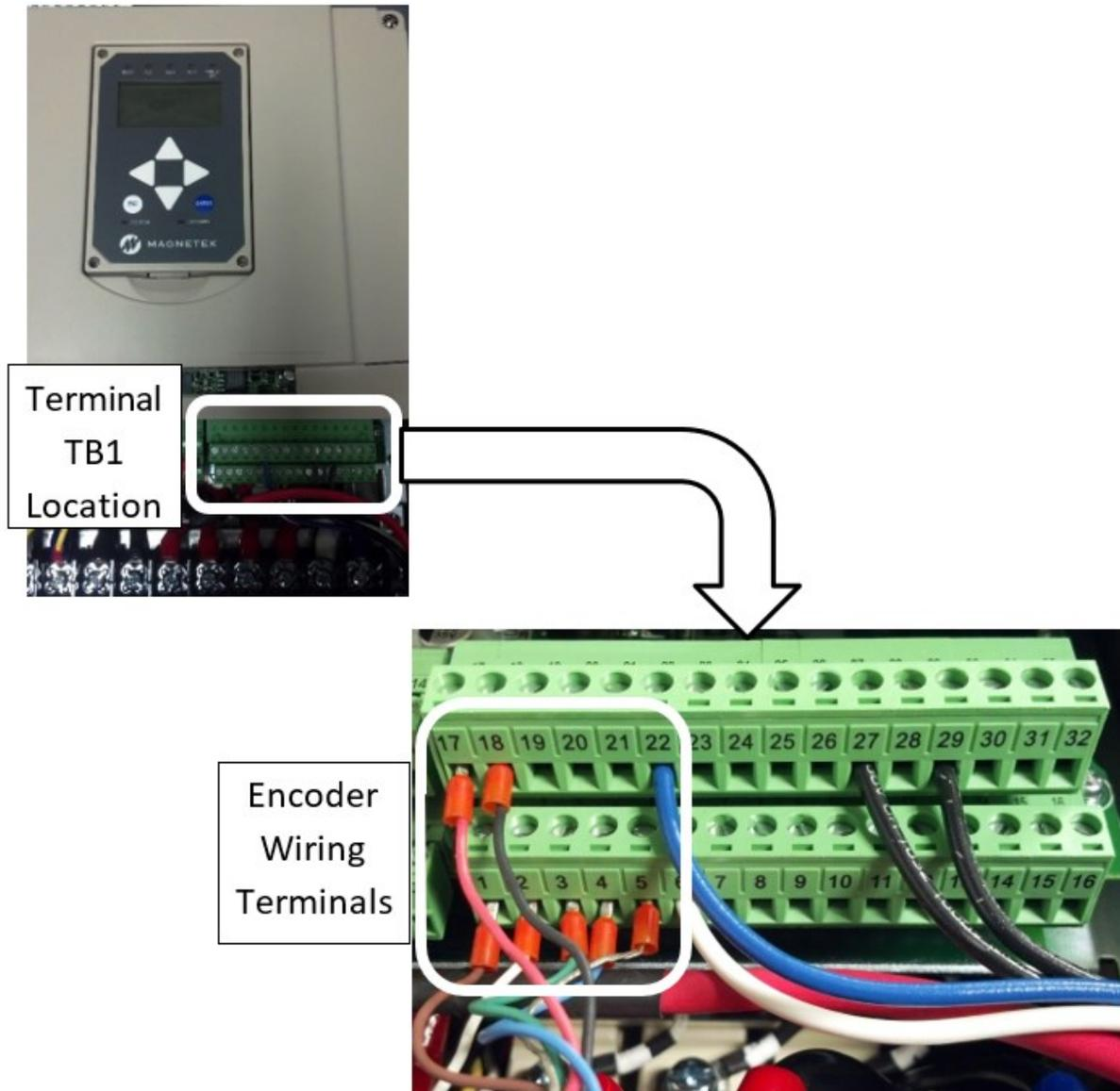
Figure 12: Encoder Terminal Location
