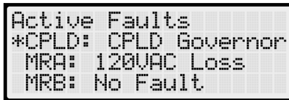
Figure 190: Active Faults Menu
