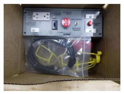
Figure 7: Inspection Box, Light Guard, 15ft CAT5
