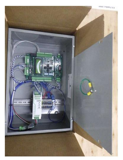
Figure 6: Controller Car Top
