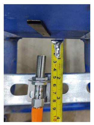
Figure 60: Mounting Proximity Sensor Assembly (Example)
