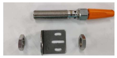
Figure 59: Proximity Sensor Assembly
