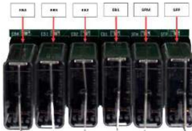
Figure 23: MR Board SR3032 Safety Relays
