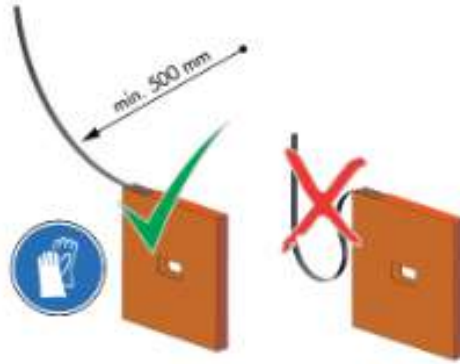
Figure 159: Tape Minimum Bend Radius
