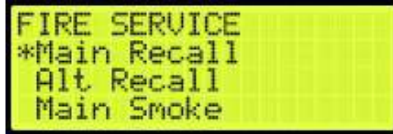
Figure 559: FIRE SERVICE Menu – Main Recall
