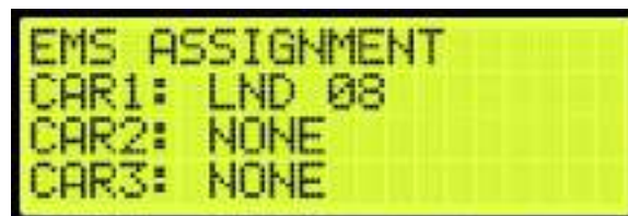
Figure 664: EMS STATUS Menu – Car 1 Assigned
