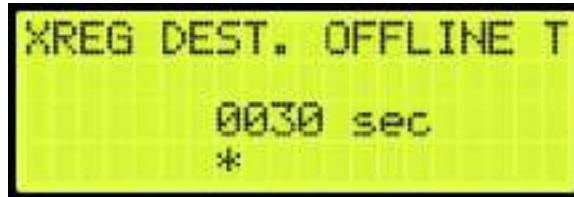
Figure 699: XREG DESTINATION OFFLINE TIMEOUT Menu
