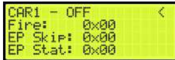
Figure 702: Fire Emergency Power Status Menu
