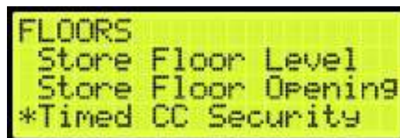
Figure 264: FLOOR Menu – Timed Car Call Security
