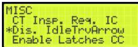
Figure 438: MISCELLANEOUS Menu – Disable IdleTrvArrow
