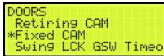
Figure 354: DOORS Menu – Fixed CAM
