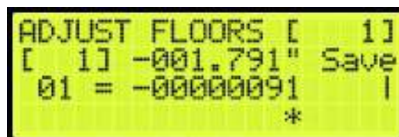
Figure 234: ADJUST FLOORS Menu – Too High
