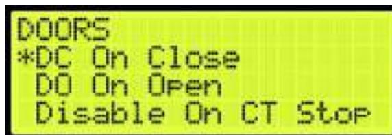
Figure 324: DOORS Menu – DC On Close
