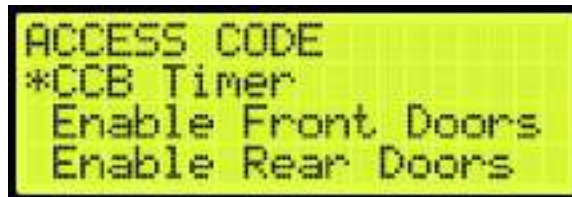
Figure 248: ACCESS CODE Menu – CCB Timer
