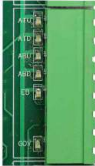
Figure 20: 120 VAC Input and Output Connector
