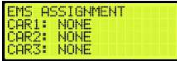
Figure 665: EMS STATUS Menu – No Cars Assigned
