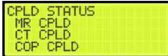
Figure 655: CPLD STATUS Menu – MR, CT, COP CPLD
