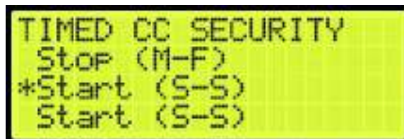
Figure 270: TIMED CAR CALL SECURITY Menu – Start (S-S)
