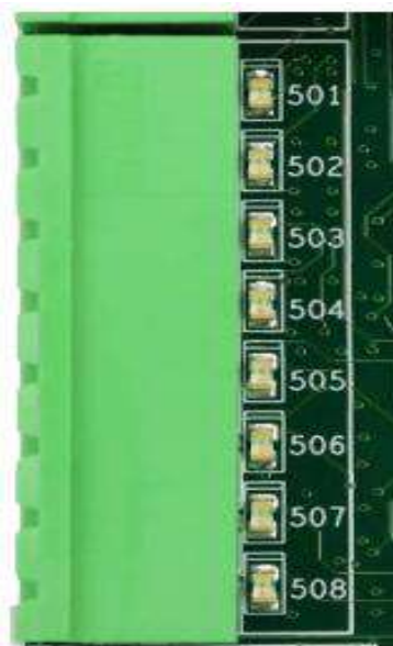
Figure 16: 24 VDC Input Connector
