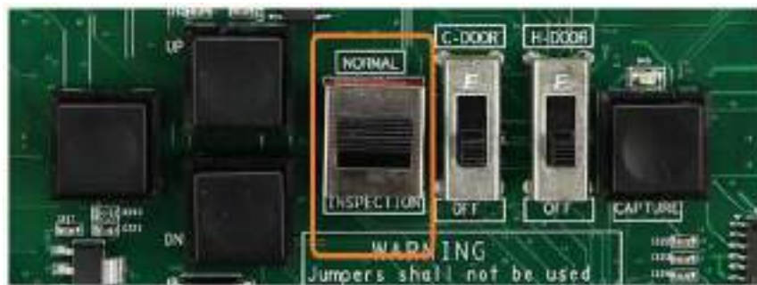
Figure 122: MR INSPECTION Switch
