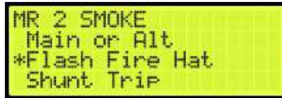
Figure 618: MR 2 SMOKE Menu – Flash Fire Hat
