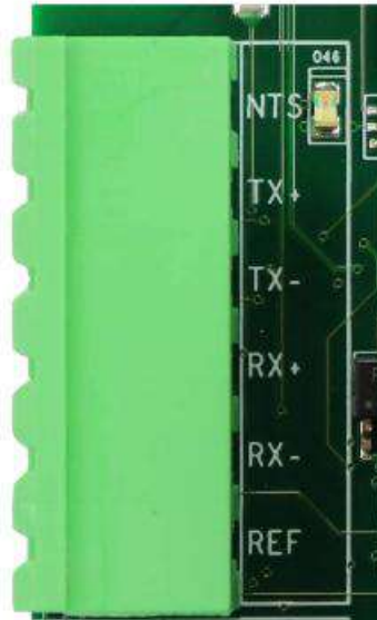
Figure 12: Drive Communication Connector
