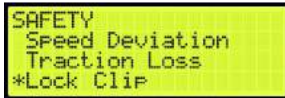
Figure 518: SAFETY Menu – Lock Clip
