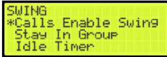
Figure 491: SWING Menu – Calls Enable Swing
