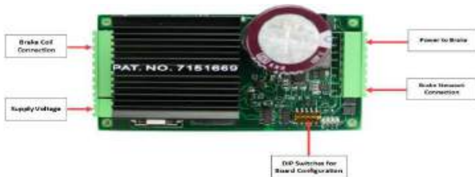
Figure 29: Brake Board SR3038
