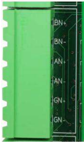
Figure 14: CAN 1,2,3 Network Connector
