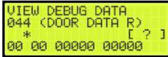
Figure 363: VIEW DEBUG DATA Menu – Rear Door
