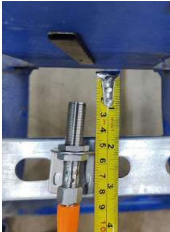
Figure 191: Mounting Proximity Sensor Assembly (Example)
