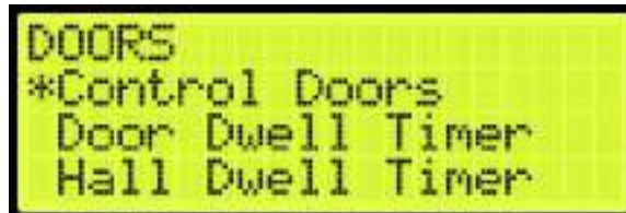
Figure 303: DOORS Menu – Control Doors
