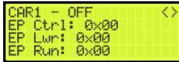
Figure 701: Emergency Power Status Menu
