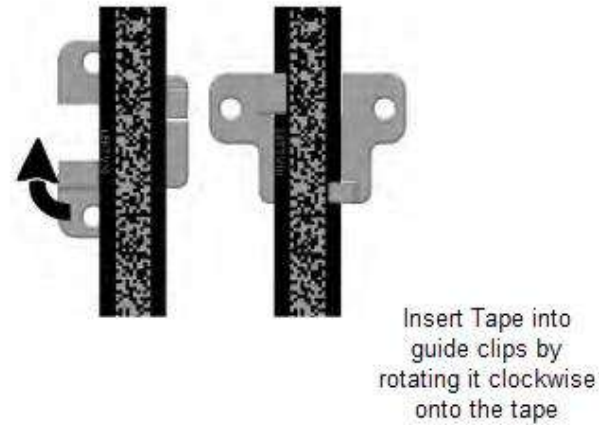
Figure 168: Tape Clip Insertion
