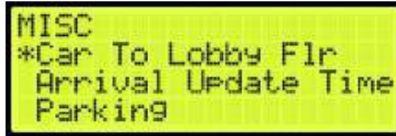
Figure 442: MISCELLANEOUS Menu – Car To Lobby Floor
