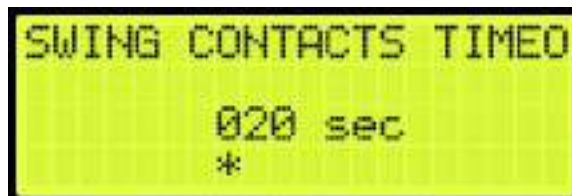
Figure 359: SWING CONTACTS TIMEOUT Menu
