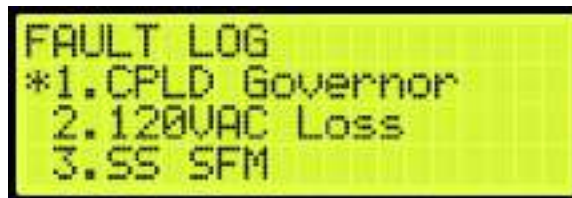
Figure 758: FAULT LOG Menu
