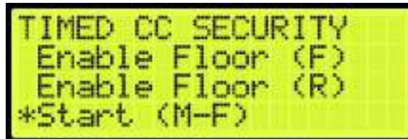
Figure 266: TIMED CAR CALL SECURITY Menu – Start (M-F)
