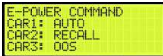
Figure 662: E-POWER COMMAND Menu
