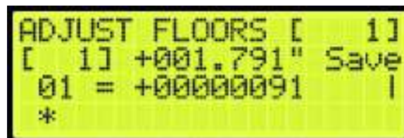
Figure 233: ADJUST FLOORS Menu – Too Low
