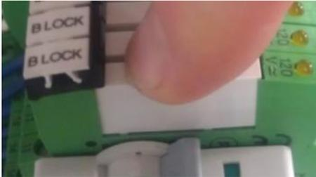
**\*\* NOTE:** If the relay you're replacing is burnt out, has been arcing or is missing a pin, you should replace the whole relay/base assembly. This will eliminate any damage done to the base from the relay terminals.
